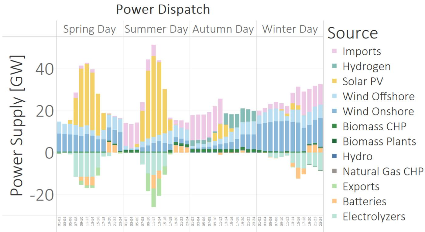
Figure 24: Power dispatch in four typical days, Central Scenario (2050)
