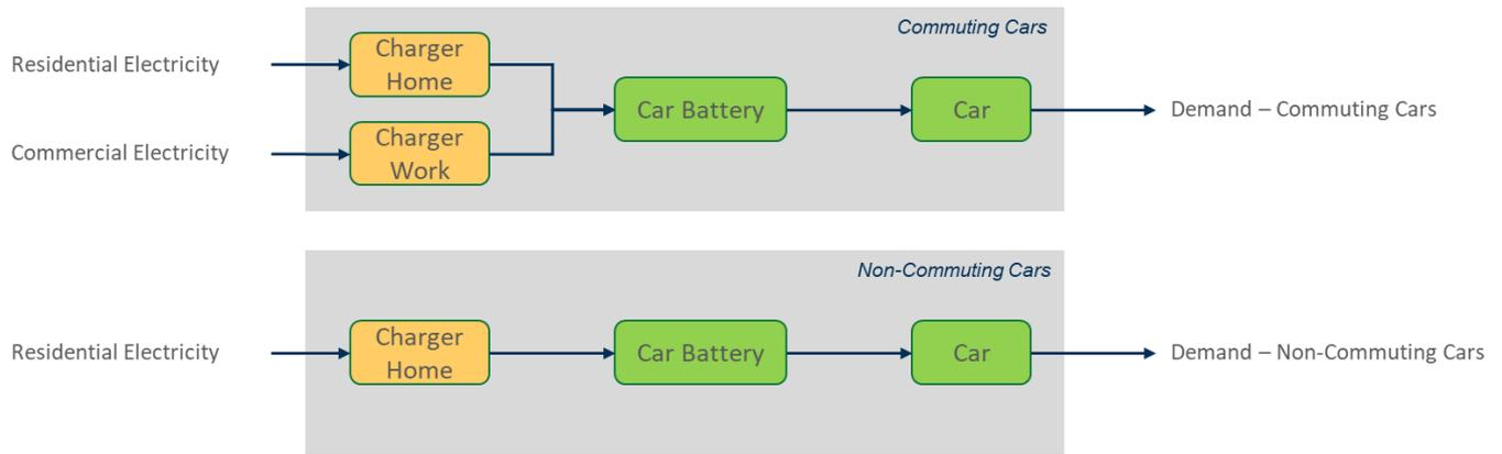
Figure 6: Scheme of charging options for EVs in TIMES-EPOC
