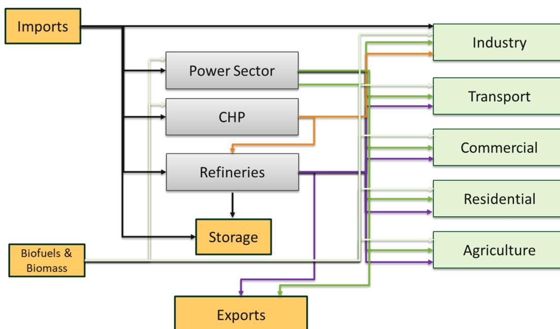
Figure 2: Simplified representation of the TIMES-EPOC model structure
